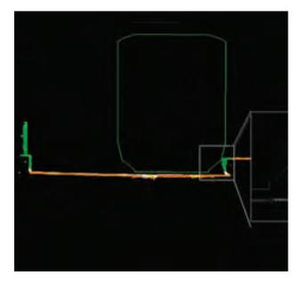
Cross-section of Lynx data point cloud, showing horizontal clearance envelope (image courtesy of SAM, Inc.).
