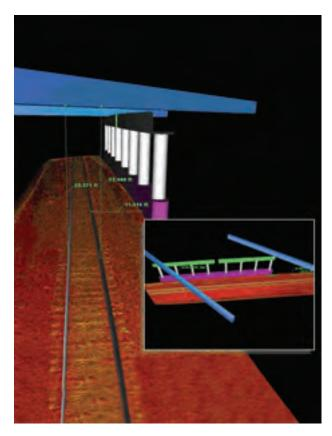
Lynx data and shape primitives of the underside of a bridge crossing the rail line (image courtesy of SAM, Inc.).
