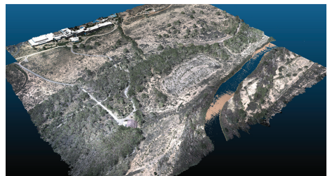
Colorized Topographic Survey collected with CLS-A.
