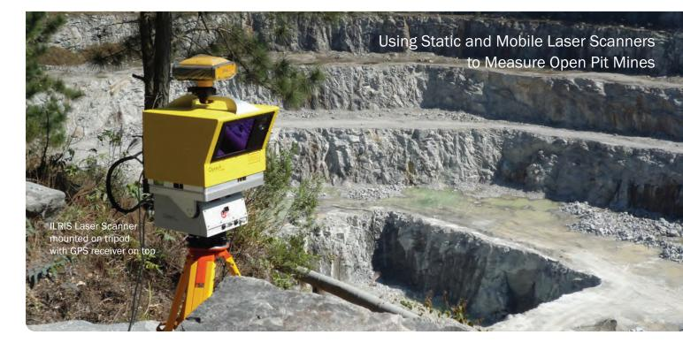
Terrestrial laser scanning (TLS) enables a surveyor to acquire massive amounts of georeferenced spatial data in a fraction of the time traditional methods require. Depending on the application, the surveyor has a choice of two TLS methods: static or mobile.
