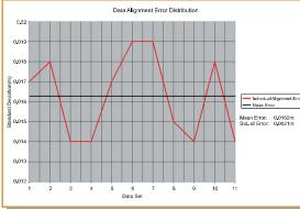
Above: Alignment statistics for all data collected. Gaussian curves indicate a normal distribution of error. Left: Magnitude of alignment error for each ILRIS-3D scan.
