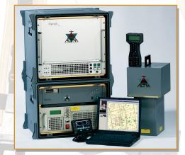
range data was seamlessly combined with GPS/inertial data to calculate the position of each measurement in a real-world coordinate system (UTM). The second set of lidar data was collected using ILRIS-3D. The characteristics of the survey site presented a challenge, primarily because of the dense city core and tall buildings surrounding the site, and because construction and security limited access to the site.
