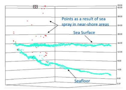
Figure 8: Original: Invalid lidar points are included in water surface measurements
