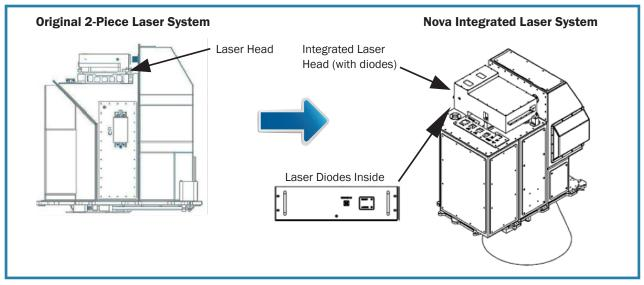
Figure 5: Single laser unit with simpler installation
