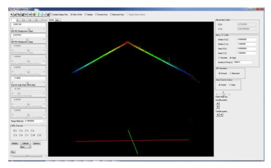
Figure 13: Automatically geo-calibrated point cloud overlaid with ground-truth data in HydroFusion 1.2, validating the calibration
