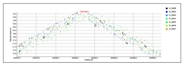
Figure 10: Uncorrected point cloud of points over a roof, colored by the flight line. Note the variations among the lines.
