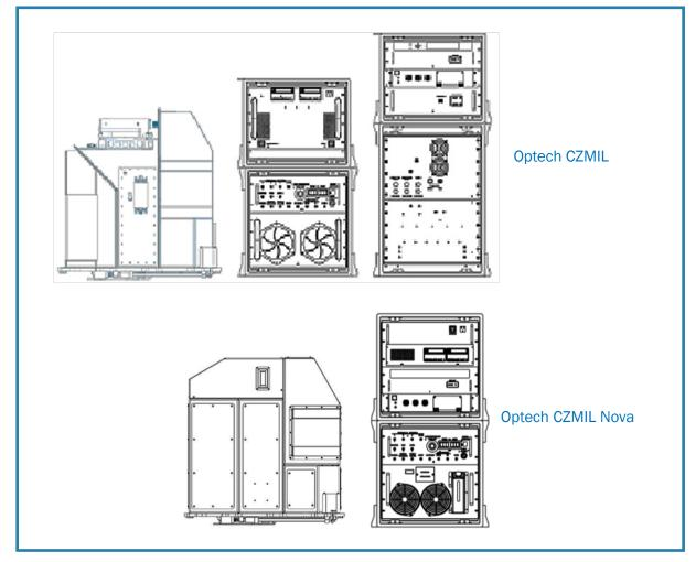
Figure 2: Smaller footprint with 30% more compact system
