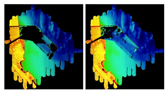
Figure 17: Survey area before processing with Turbid Water Module (left) and after processing (right)
