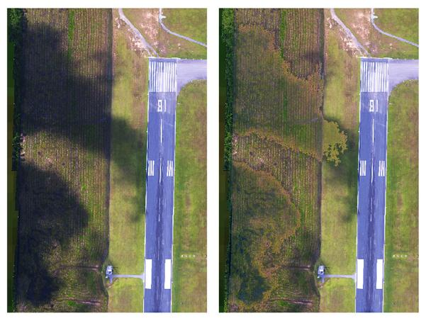
Figure 15: Example 2: Color balancing of image mosaics in HydroFusion 1.2, before balancing is applied (left) and after (right)
