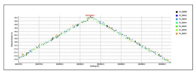
Figure 11: Automatically geo-calibrated points over the roof, colored by the flight line
