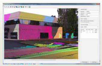
Extracted lidar planar patches projected to the imagery for visual inspection of the co-registration between the two datasets.
