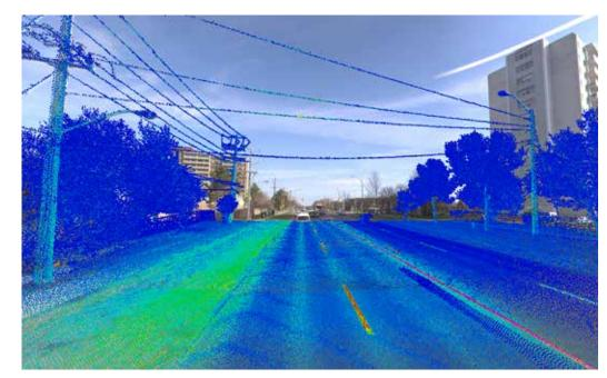
Optech LMS integrates both lidar and image sensor processing methods into a single workflow platform, enabling comprehensive sensor calibration and accuracy quantification
