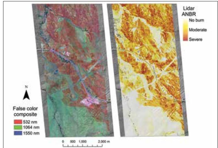
of a fire using the ALTM Titan to compute the ANBR, and then potentially use a satellite-based NBR product to extrapolate the total peatland soil loss over the entire fire area.
