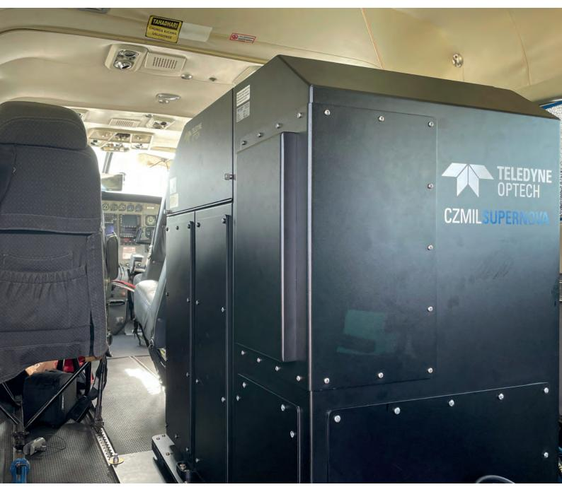
▲ CZMIL Supernova installed in a Cessna 208B Caravan aircraft.
